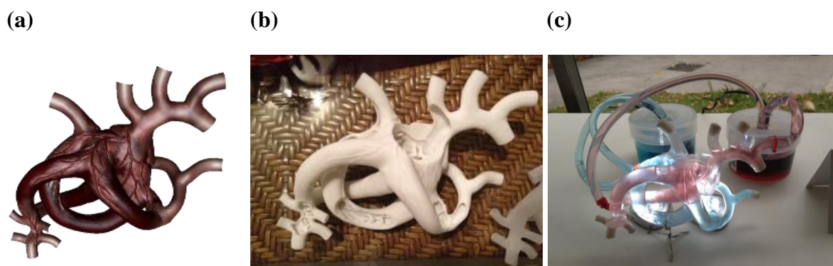
Figure 8. Heart provocation models by MA student Kaecee Fitzgerald (a) CAD model; (b) 3D print from the CAD model; and (c) heart in action showing flow.
