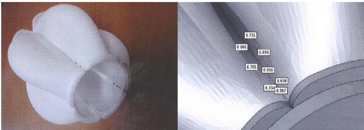
Figure 7. Example of a build problem (a) and the Shapeways problem report (b)
