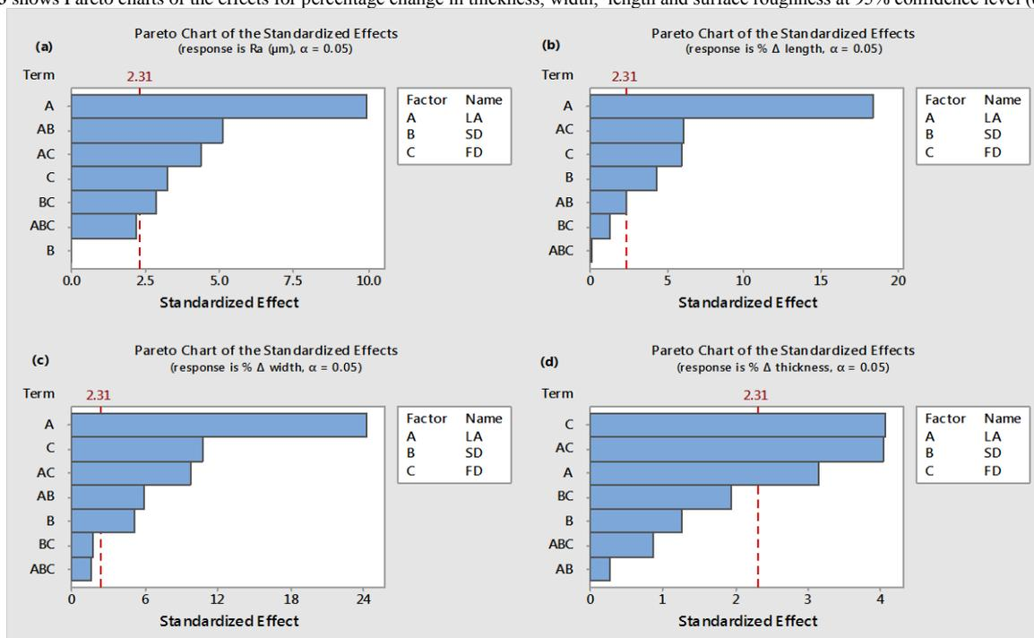
Figure 3 Pareto chart of standardized effects for (a) Surface roughness (b) % change in length (c) % change in width (d) % change in thickness
